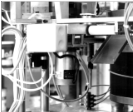
Rotary table with step motor.
