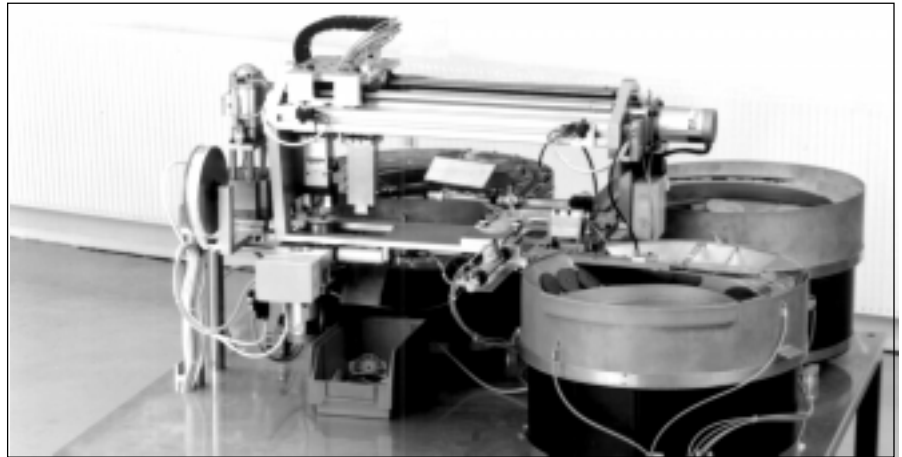
The complete handling and assembly machine for filter dispensers.
